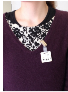
FIG. 2. The RFID tags were worn on the chest of the participants, enabling communication with other tags when two participants were facing each other.
