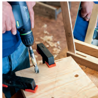
USED IN STEP 6 The brad point bit has a raised centre point that digs into timber so it won't skip when drilling.
