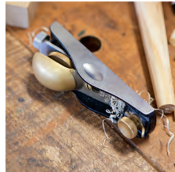
USED IN STEP 4 The block plane is smaller than a smoothing plane and is used for fine shaping.
