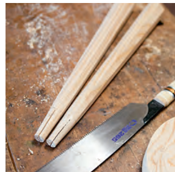
USED IN STEP 9 The Japanese handsaw cuts on the pull stroke, unlike other saws that cut on the push stroke.
