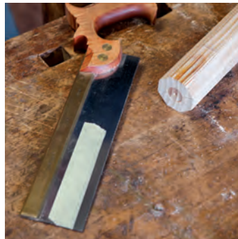
USED IN STEP 3 A tenon saw is a fine-toothed saw with a rigid blade used for cutting across timber.
