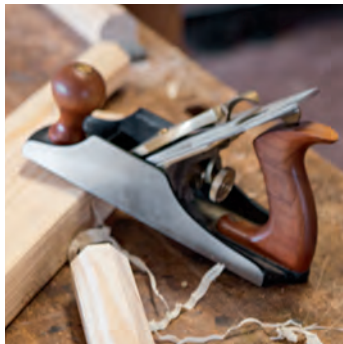
USED IN STEP 1 The smoothing plane will help give a finer finish to timber after a rough shaping.
