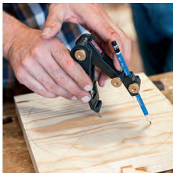
USED IN STEP 5 The compass (remember geometry class?) is used to draw a circle from a central point.
